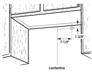
**To wire through rear,** mark a line 7-1/2" from the right of the centerline on the wall. Mark the point on this line that is 1-3/8" from underside of cabinet. Drill a 1-1/4" diameter hole through wall at this point.
